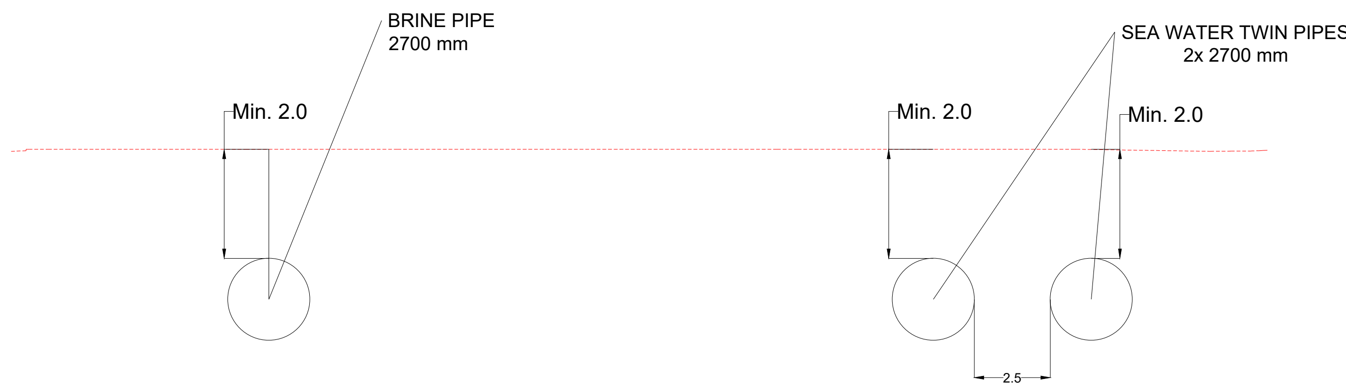
40m DLS R.O.W LOCATION OF THE PIPES WITH RESPECT OF THE ROAD
